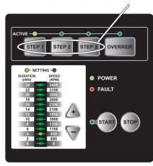
The enviroMAX user interface has a "key lockout" feature to prevent unwanted changes to the settings.
