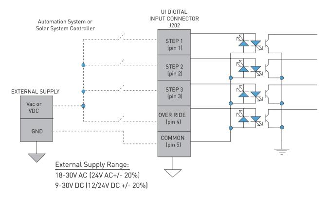
Figure 6: Wiring Diagram for Automation Control System Inputs
