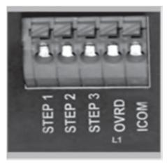
Figure 7: Automation Control System Input Connector
