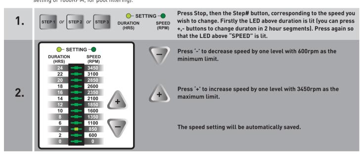
**Note:** If power is cycled to the pump and the user does not press the STOP key, the pump will automatically start and run the programmed default schedule shown in the chart above. This feature ensures that the pump will re-start in the event of a power outage. The pump will start on STEP 1.
