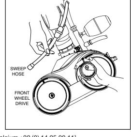
If the RPM is more than 32, at the Wall Fitting, unscrew the Pressure Relief Valve slowly until the RPM falls between 28-32.
