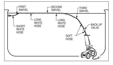
two (2) mender nuts (ED15/LLD15PM). Attach extra white (hard) hose between soft hose and existing white (hard) hose, using floats, swivel and mender nuts. Divide extra white (hard) hose overage by three (3) this time to keep all white hoses the same length.
